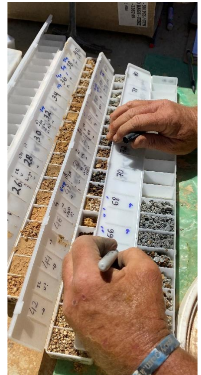
Figure 1 – Annotating chip trays from an RC drill hole on site at La Mascotte. The geologist is annotating the trays for signs of alteration and mineralisation.
