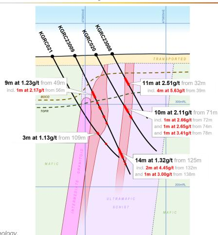
Cross section at Providence, showing KalGold and historic drilling and interpreted geology.
