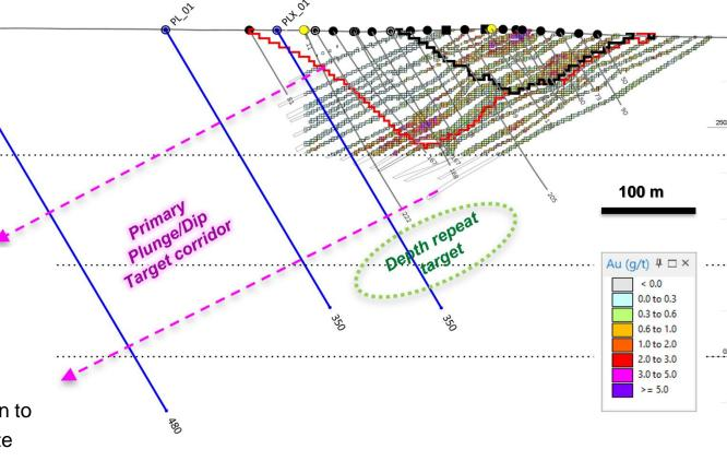
Cross section at La Mascotte through the block model generated for the JORC resource estimate. Conceptual deeper drill holes are shown that could substantially increase the resource if successful. This and other programs are being evaluated.
